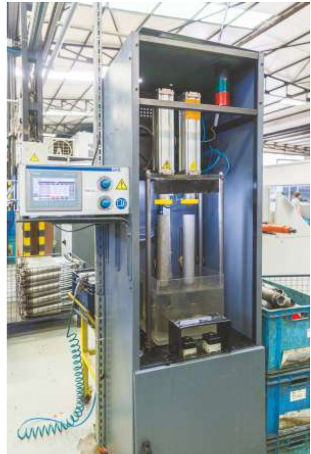
Leakage Test (Welding Parts)
