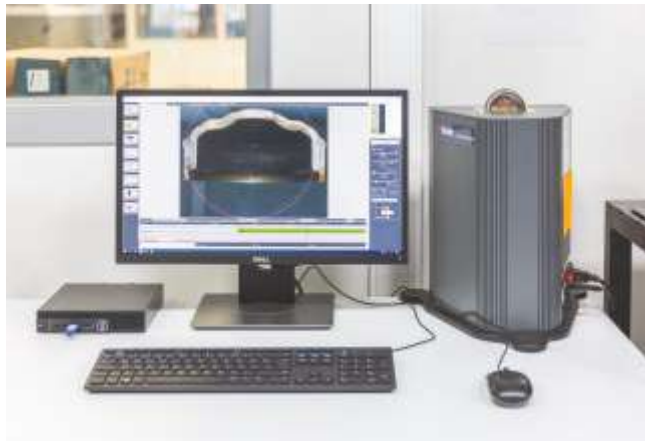
Welding Penetration Test
